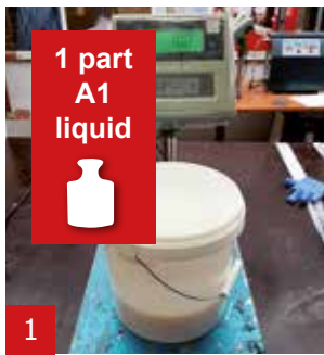
1 Calibrate the scale and weigh 1000 g A1 liquid...
