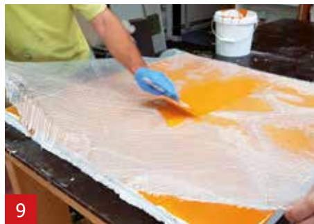
9 Smoothen the triaxial fibre with the spatula from the center.
