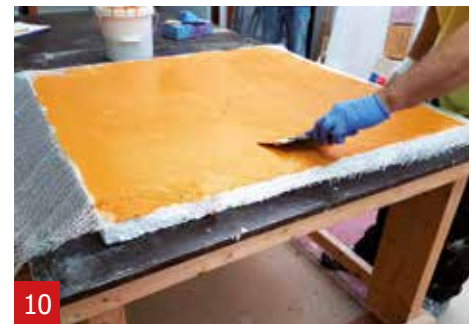
9 Smoothen the triaxial fibre with the spatula from the center.
