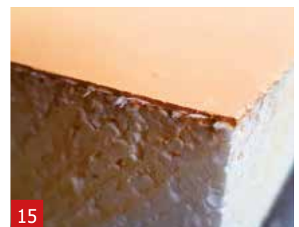
15 Final result , a strong panel, coated with a thin layer of A1.
