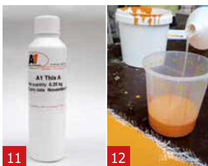
11 Add 1% of Thix A to the remaining A1 and stir well with a stirring rod. The A1 becomes thicker.
