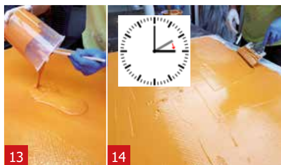
13 Apply this mixture with the spatula on the surface of the panel to create a smooth finish layer. Let it cure \pm 1 hour.
